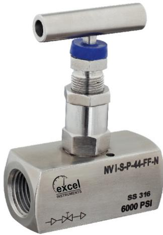
Type needle valves with hard seat are designed for use on applications requiring complete isolation or throttling of the media. The conical metal tip (Stem Type CT) press fitted ensures perfect alignment for positive bubble tight shut-off. Available with end connections in sizes from 1/8" to 1" and a wide choice in connections of female screwed, male screwed, male to female screwed or socket weld.
