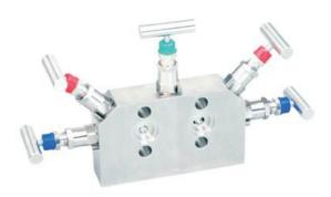
Coplanar mounting Five Valve Manifold with drain plugs. This manifold has two isolating valves, one equalizer valve & two vent Valve. When assembled to transmitter has the advantage of compact size with easy for operation in minimum space. The direct mounting facility to the base of the differential pressure transmitter result in less leakage points and more accurate measurements.
